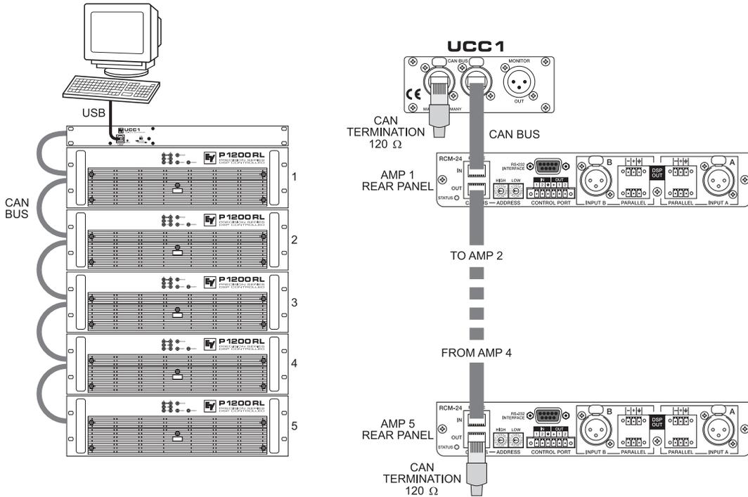
System with 5 amps and one UCC1 / PC at the beginning of the bus
